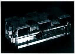
All Tyler Research horizontal systems may be run in both submarine and agarose wick formats. The latter is particularly useful for high resolution separation of RNA fractions, and the sliding gate system operates within a modified J-wick assembly that permits rapid gel preparation and safe disposal of potentially toxic gel waste.
